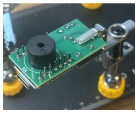
Then test that it works BEFORE you put it in the case. Once it is in the case it will not come back out easily. Fix any solder joints if you have issues. The arduino is preflashed with the correct firmware so no need to do that during assembly.
