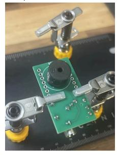
Solder the buzzer leads from the other side, and snip them off once soldered. Make sure the buzzer is flush pressed against the pcb. You might have to hold it together with one hand or clamp and solder with the other. If it is not flush, it won't fit in the case later.
