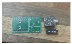
Snap the aux jacks into the PCB, being very careful not to bend the pins when inserting it into the arduino. They should hold themselves in well, but make sure they are firmly flush to the PCB when soldering them from the other side.
